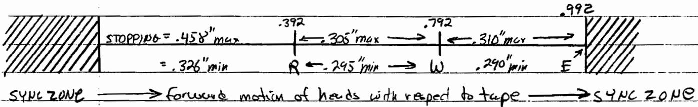
Shown above is a first pass at the positions of the Read (R), Write (W) and Erase (E) heads when they come to a stop following a forward read or read after write. After the Read head exits the sync zone it takes from .326" to .458" to stop. The ranges on the ranges on the mechanical spacing of the 3 heads is also given.
